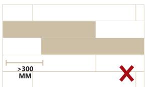
The longest side should be staggered no more than 300mm when laid in running bond.
